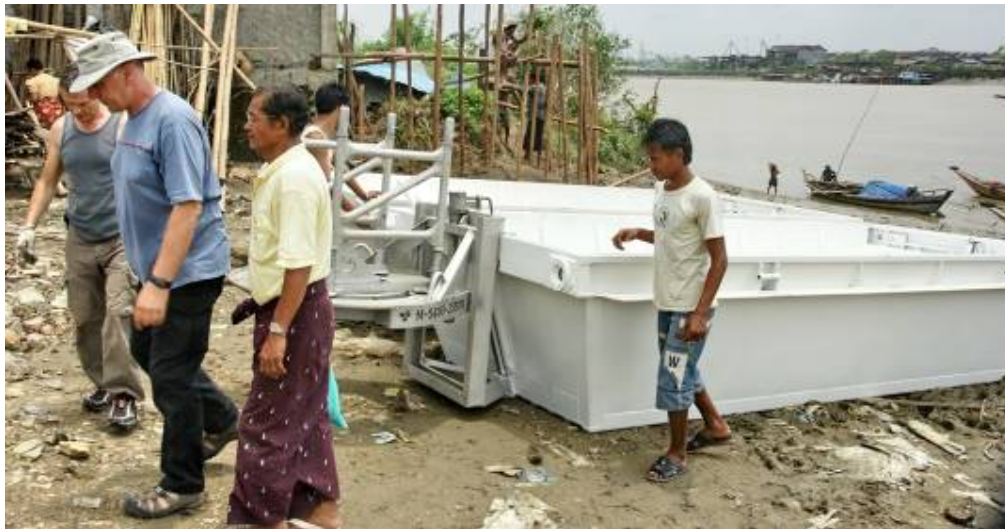
Stuart Kingsley and Brian Davison with two of the river boat hulls - The stern assembly can clearly be seen, ready to receive a 40 HP Mercury Mariner outboard propulsion unit. The whole units, including the specially designed high-torque propellers can be raised or lowered from inside the hulls when the boats enter shallow waters. Hlaing River, 19 th May, 2008
