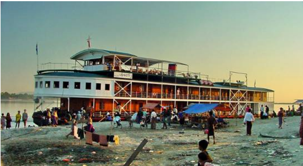
The Pandaw II moored beside the Ayeyarwady River - Built in Yangon's shipyards in 2001 for the Irrawaddy Flotilla Company, Paul Strachan has donated this 180 foot, 34 foot beam vessel for use by Save the Children as a mobile hospital ship in the Delta. With 24 double cabins, the ship is a classic triple deck river vessel with a shallow 3 foot draft for navigating the Irrawaddy between Yangon and Mandalay
