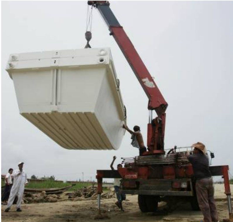
Unloading one half of an aluminium river boat by crane beside the Hlaing River outside Yangon ready for assembly & river trials along the Hlaing River – Monday morning, 19 th May 2008
