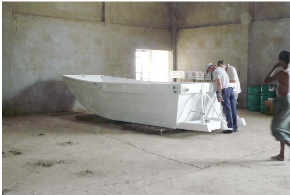
The forward bow half of the 14 motorised 40 foot aluminium boats showing the mid-ship bulkhead where the rear after section bolts the whole craft together. 7 of these boats will arrive in Patheingyi by road this afternoon, ready for assembly or transshipment down to the Delta
